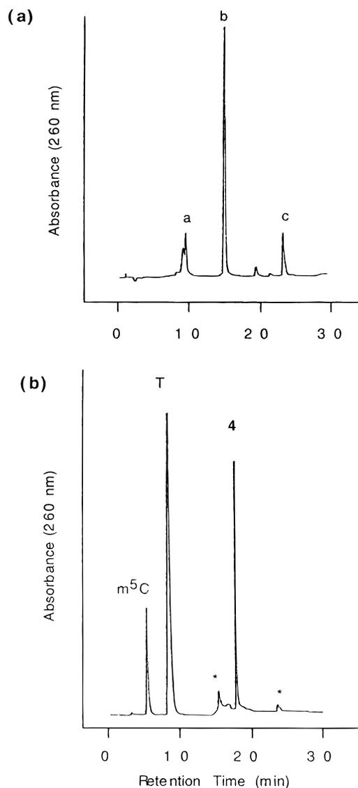
**Figure 1.** (a) HPLC analysis of the crude reaction mixture obtained after ammonia deprotection of the conjugate **8**. a: 15-Mer polypyrimidine DNA sequence, b: Hoechst–15-mer conjugate, c: Hoechst–hexa(ethylene glycol) derivative **4**. (b) HPLC analysis of the snake venom phosphodiesterase/bacterial alkaline phosphatase digest of a DNA 15-mer conjugated to the Hoechst derivative **4**. \* marks unidentified contaminants in the buffers.
